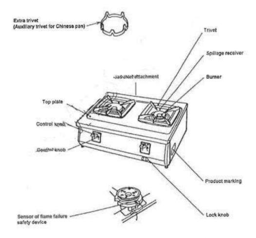
Figure 7. Part of table types appliances with two cooking burner
