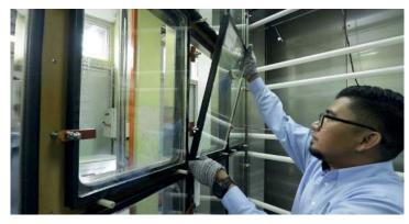
IGU, more commonly known as double-glazed glass, consists of two-three glass window panes that is separated by inert gases in order to reduce heat transfer across a part of the building envelope. As a result, buildings can see a reduction in HVAC (heating, ventilation and air-conditioning) usage which is a comfort to any company's annual savings and energy consumption rate.
